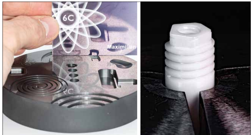
Fig. 2 Cut demo-part made of silicon carbide (l.) and cut M3 inner thread, M6 outer thread and hexagon head screw made of zirconia (r.)
