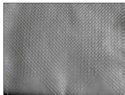
Fig. 3 Fabric with diagonal reinforcements (Open Riet fabric)
