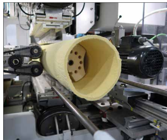
Fig. 2 Production of a nonwoven tube at TFK
