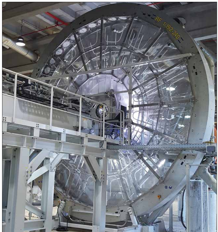
Fig. 9 Radial braider for manufacture of textile preforms with a diameter up to 57,5 cm installed at TFK
