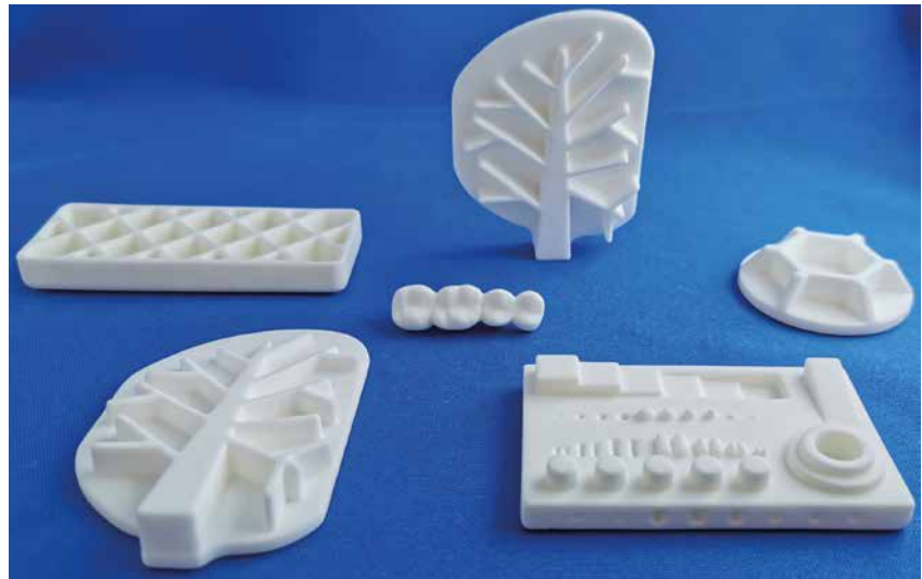
Fig. 3 Examples of printed alumina parts (f.l.t.r.): a rectangular 3D-grid (75 mm × 29 mm × 10 mm), two laser mirror-like structures (66 mm × 47 mm × 11 mm), a dental bridge (35 mm × 12 mm × 11 mm), a rotor-like structure (41 mm × 11 mm), and a test artifact adapted from NIST (66 mm × 41 mm × 10 mm)
