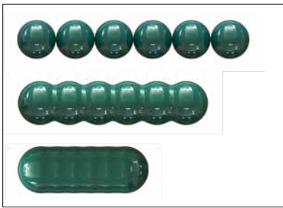
Fig. 1 Transition from single droplets to line structure using defined droplet fusion factors
