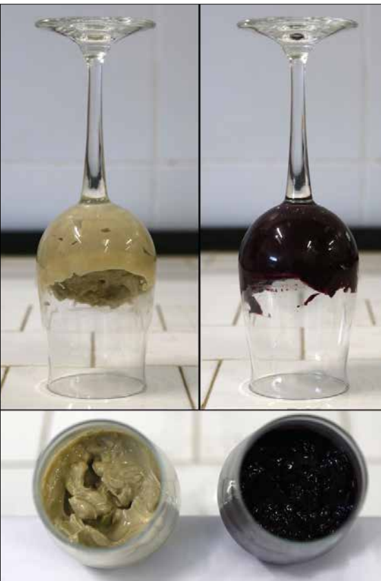
Fig. 4 Example for the high viscosity that can be obtained with DCF (red and white wine lees) [5]
