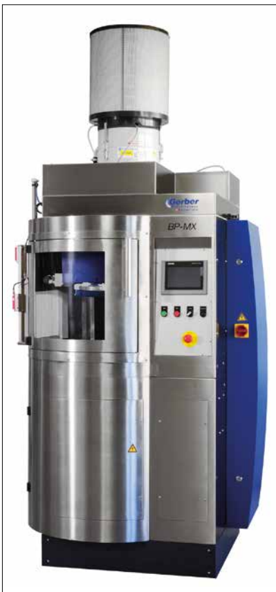
Fig. 1 The BP-MX brush polishing machine
