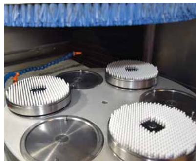
Fig. 2 Ceramic axles in the BP-MX brush polishing machine
