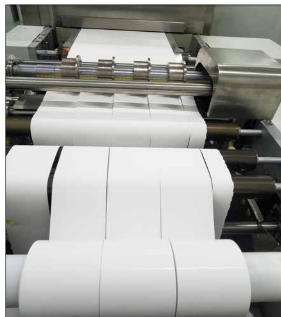
Fig. 1 Continuous production of green tapes in the SEDAL facilities
