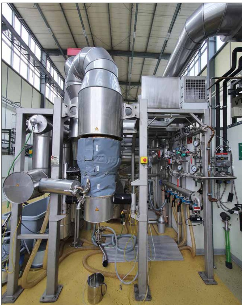
Fig. 1 Photograph of a newly developed, high temperature fluidized bed coater for spray pyrolysis and coating of Li-containing compounds on battery materials
