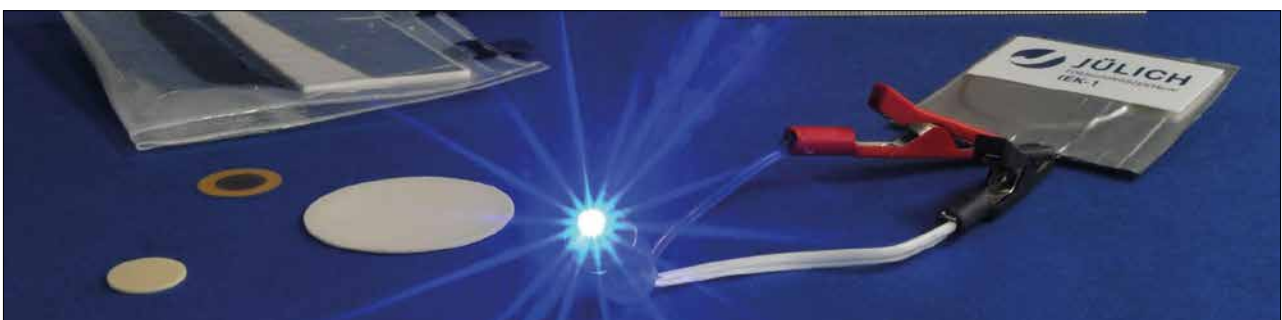
Fig. 5 Demonstration of an all-solid-state pouch cell with a sintered LLZO separator (l.), a composite LCO + LLZO cathode and a metal Li-anode operating at room temperature
