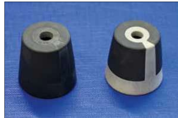
Fig. 3 Sintered 2C-nozzles in two material combinations
