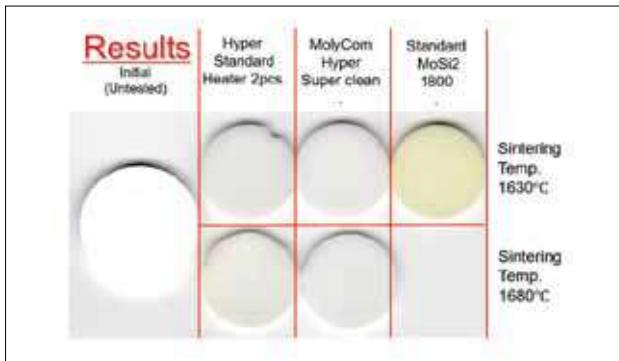
Fig. 6 Color changes from different heating element qualities
