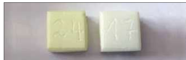
Fig. 9 Sample 24 was sintered on a closed saggar (muffle); sample 17 was inside the saggar in the same firing run in a contaminated furnace
