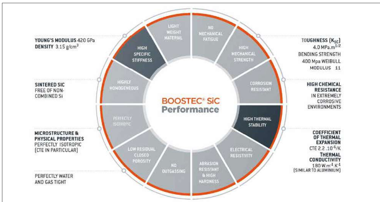
Fig. 3 Typical Boostec® SiC properties
