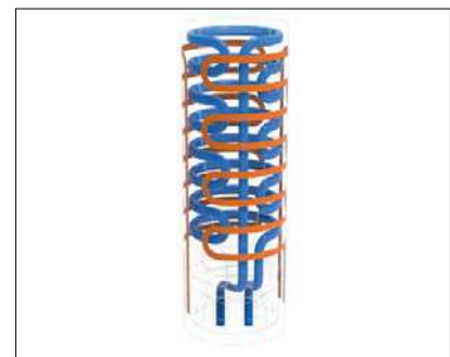
Fig. 2 Design of the cooling (blue) and heating (orange) elements
