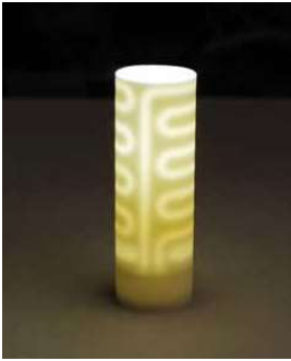
Fig. 4 Sintered CerAM VPP component with internal cooling channels
