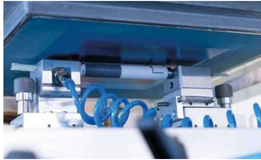
Fig. 5 Screen printing on tubular component
