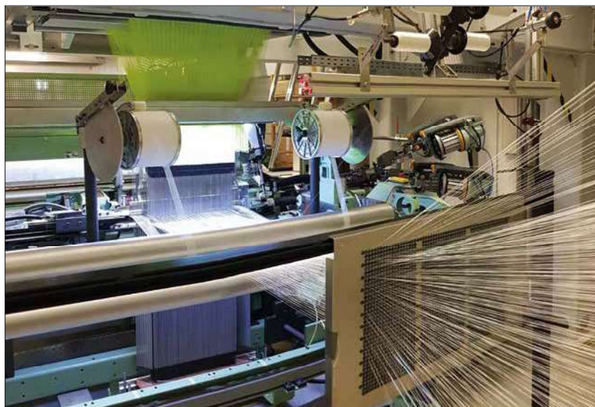
Fig. 2 Weaving of OxCeFi fibres
