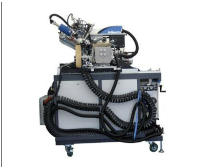
Fig. 4 New beamline PLD system for in situ synchrotron diffraction (source: SURFACE)
