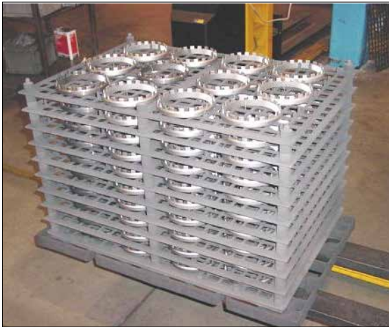
Fig. 5 Fully loaded C/C fixture, plate design, with internal gears, 10 layers (3-dimensional), 5 mm x 500 mm x 600 mm, 120 parts [6]
