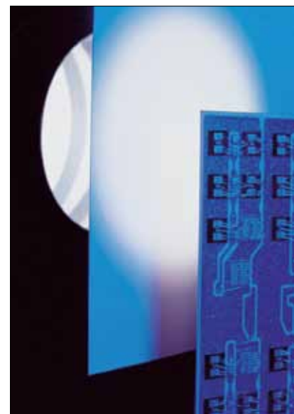
Fig. 5 Thin ZTA substrate for heat sinks produced by tape casting
