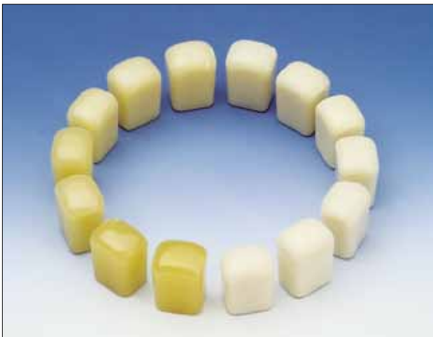
Fig. 6 Glass ceramics with adaptable translucency and colour for aesthetic dental restorations
