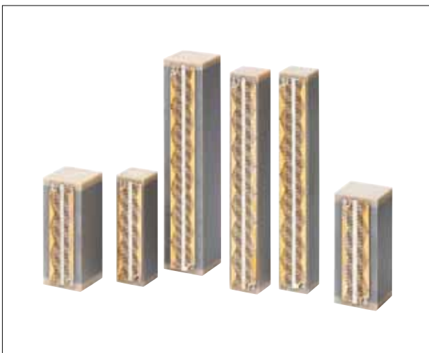
Fig. 6 Patented, meander-shaped external electrodes: stable electric contact even under extreme dynamic stresses (Source: PI Ceramic)
