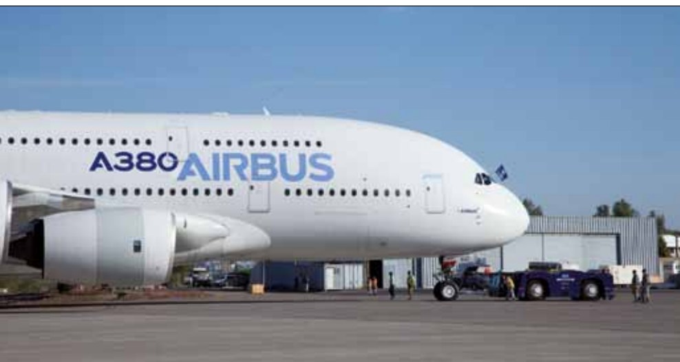
Fig. 1 The largest passenger airplane currently in series production is the Airbus A380. Its doors are large and too heavy for manual closing (Source: Airbus)
