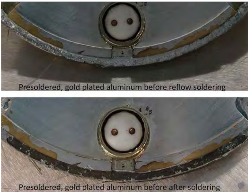
Fig. 9 Aluminium pretreated with active solder before and after reflow soldering
