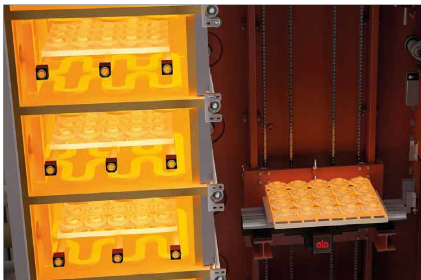
Fig. 1 Multiple-chamber vacuum-heat treatment module ALD SyncroTherm® (ALD, Hanau)
