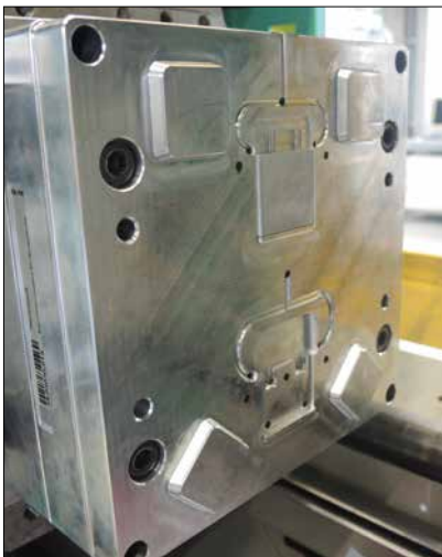
Fig. 8 Mould for producing insulator and conductor component
