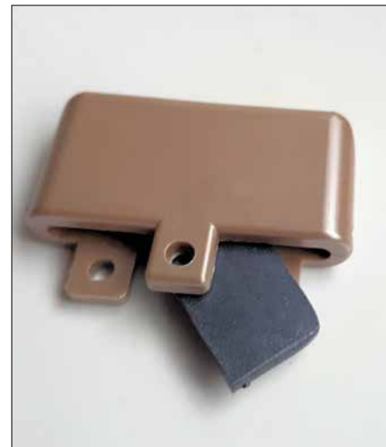
Fig. 10 Sintered TiO 2 -insulator and TiO x -conductor, ready to be joined by an adhesive
