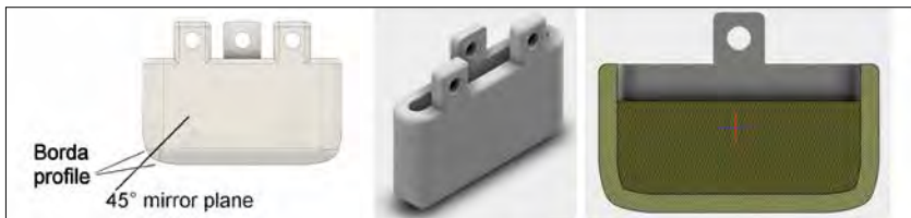
Fig. 6 Design of the plasma electrode with mirrored Borda profile left and right
