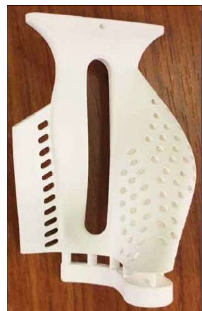
Fig. 6 Core after printing and firing
