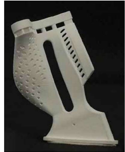
Fig. 10 The production of cores is optimized thanks to 3D printing
