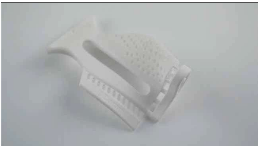
Fig. 1 A new generation of foundry cores produced by 3D Printing
