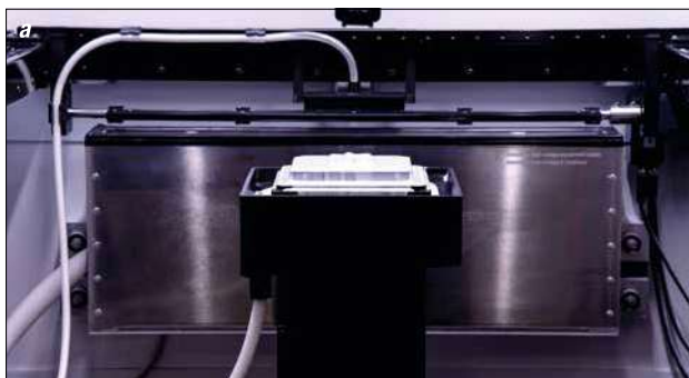
Fig. 3 a–b Views of the CeraMax Vario V900's build platform, offering a building envelope up to 250 mm x 250 mm x 290 mm, showing a finished green part after being elevated from the vat
