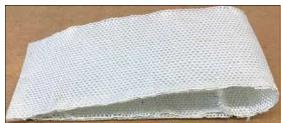
Fig. 8 First preform produced on a laboratory loom
