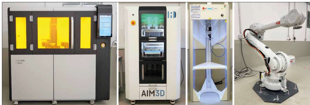
Fig. 4 The equipment available at 3DK for creating printed parts from left to right: CeraFab Multi 2M30 from Lithoz GmbH/AT; ExAM 255 from Aim3D GmbH/DE; WASP 40100 Clay delta printer/IT; 6-axis industrial robot from ABB Automation GmbH/DE
