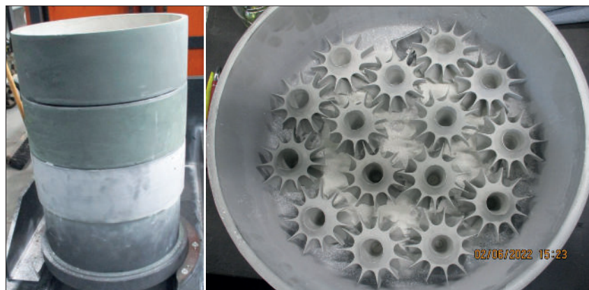
Fig. 10 NSN sintering crucibles for GPS of silicon nitride turbine wheels: crucible stack (left); view into a crucible (right)
